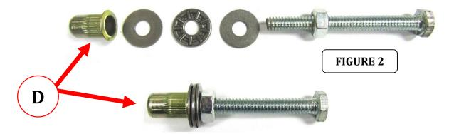
**Step-4** Place the rivet-nut with the attached tool components into the enlarged hole in one of the tabs. Use a 7/16" wrench to hold the nut, and tighten the bolt using a 7/16" wrench or socket and ratchet. Continue tightening the bolt until the rivet-nut is fully compressed and no longer spins then remove the tool components, (FIGURE 3). Repeat for the enlarged hole in the remaining tab.
