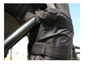
3. Now install the tension straps to hold the top tight. The strap hooked end attaches to the tub, goes over the third bow (last bow) and back to the buckle. Tighten this strap snug. Pulling down on the bow a little and tightening the buckle will insure a snug top.
