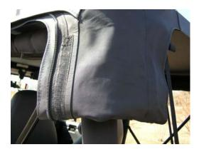
2. Once the fourth fold is done the sail panel will look like above. Place the pocket under the sail panel and insert the panel into the pocket. Now strap the pocket to the roll bar. The top strap (or both) goes over the top bow as shown in the photo below.
