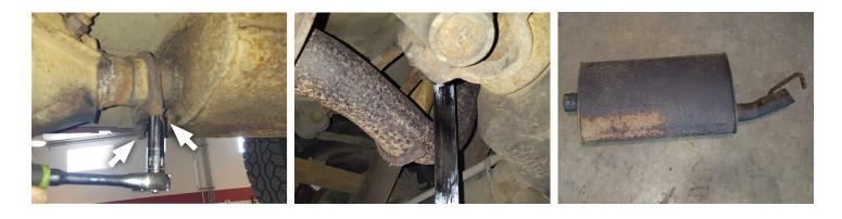
4. Remove bolts (x2) and hanger mount near exhaust exit then remove tailpipe. Retain bolts for later use.
