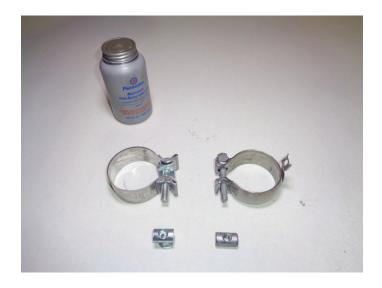
www.flowmastermufflers.com Technical Support (866) 464-6553  Place clamp (9) onto inlet pipe (1) then connect it to catalytic converter. Tighten clamp just enough to allow for adjustment.
