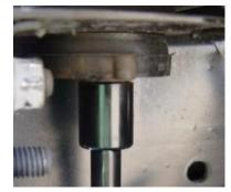
Step (2) Align inner and outer mounting holes with the rear frame cross member. (2 outside of frame rail, and 2 inside frame rail for each side). Use the 10mm bolt washer, and nut. Torque bolts to 50 ft-lbs.
