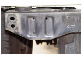
Drill holes into rear cross member. WARNING ... BE VERY CAREFUL WHEN DRILLING
