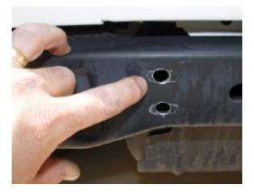
Attach the hitch with the (4) 10mm bolts, flat washer, lock washer and nuts supplied for each side. Tighten to 45lbs (Total of 8). **NOTE: ON 97-2006 Wranglers there might be a tight fit between the rear cross member and the fuel tank. A second person will help with installation.**
