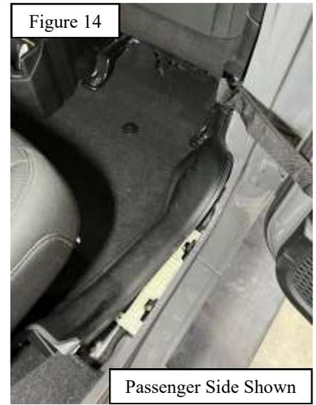
**Step 12:** With the panels removed, on the passenger side, lift carpet back to expose the drain hole under the carpet.
