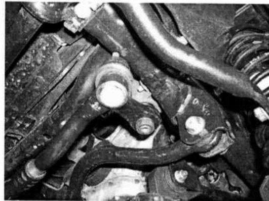
Disconnect front track bar from axle. It is not necessary to disconnect it from the frame as shown.
