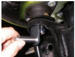
**Note:** Factory offset wheels with larger tires may rub on the QD link. Different off-set wheels or wheel spacers will be required.
