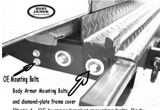
Photo 4 - OE bumper bracket mounting bolts, Body Armor bumper mounting bolts and diamond-plate frame filler plate (uses 1 bumper bolt each side).
