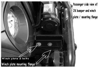
Photo 2 - passenger top-view winch plate mounting.
