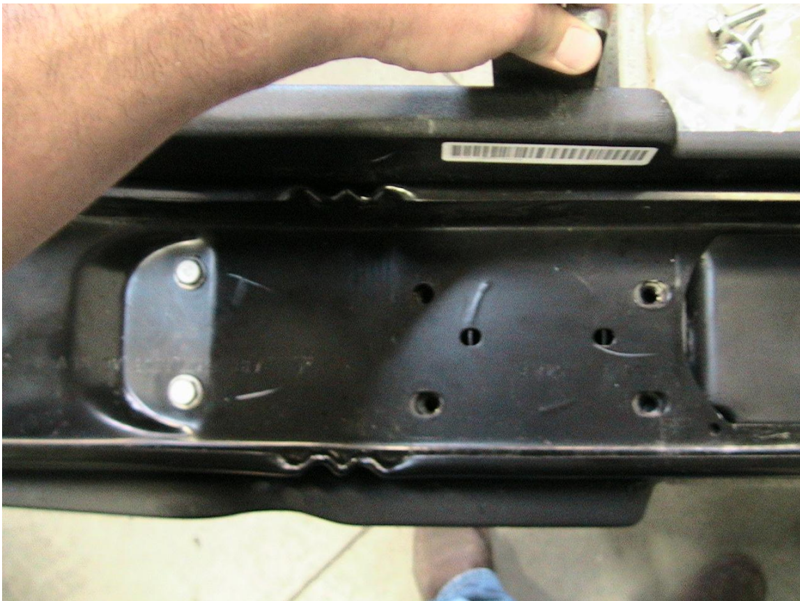
Figure 6: Front Bracket must fit flush to steel bumper
