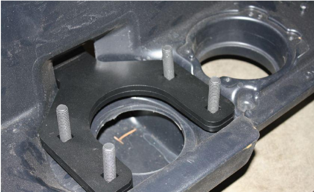
Figure 5: Front Frame Bracket fitment into plastic bumper
