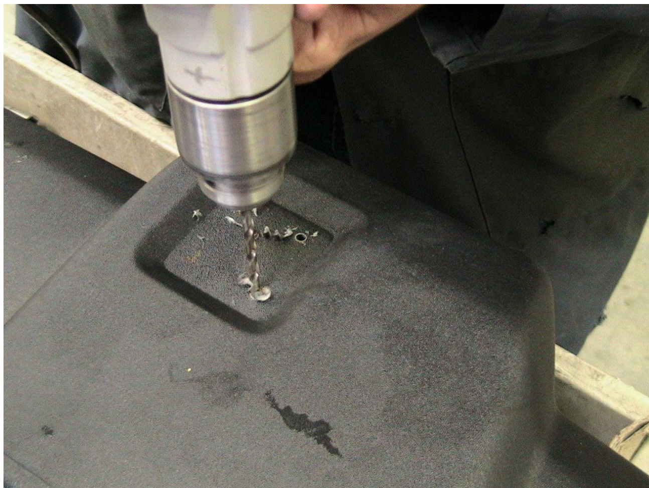
Figure 3: Drill corners of tow hook cutout
