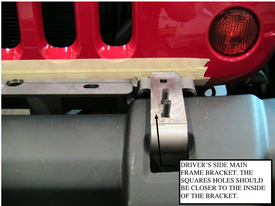
Figure 9: Driver's side main frame bracket
