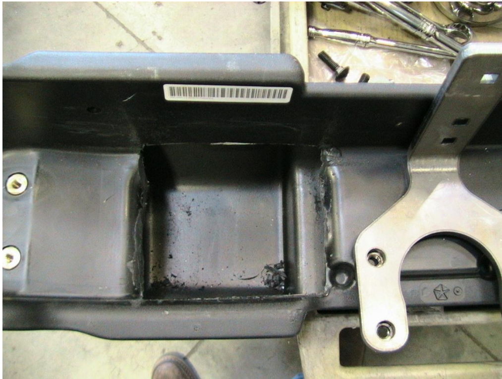
Figure 7: Cutout of inside of plastic bumper
