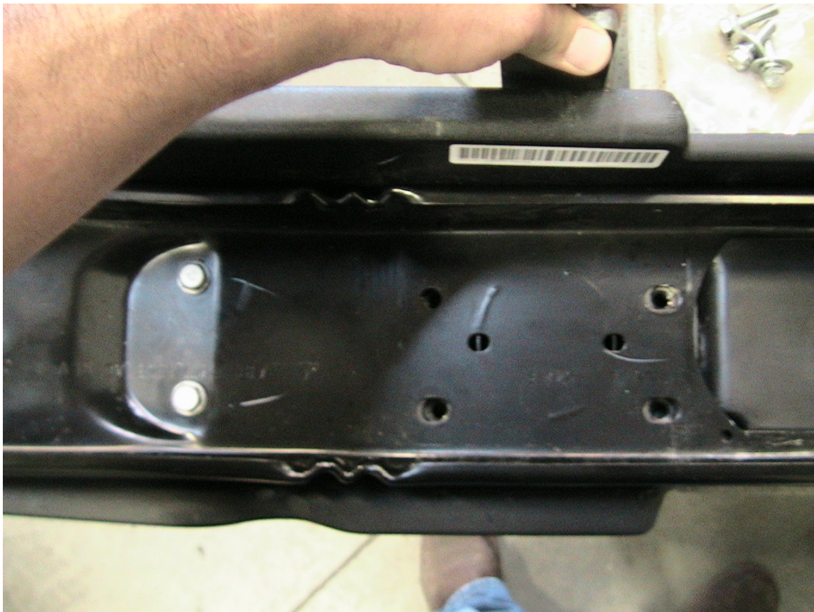
Figure 6: Tow hook must fit flush to steel bumper
