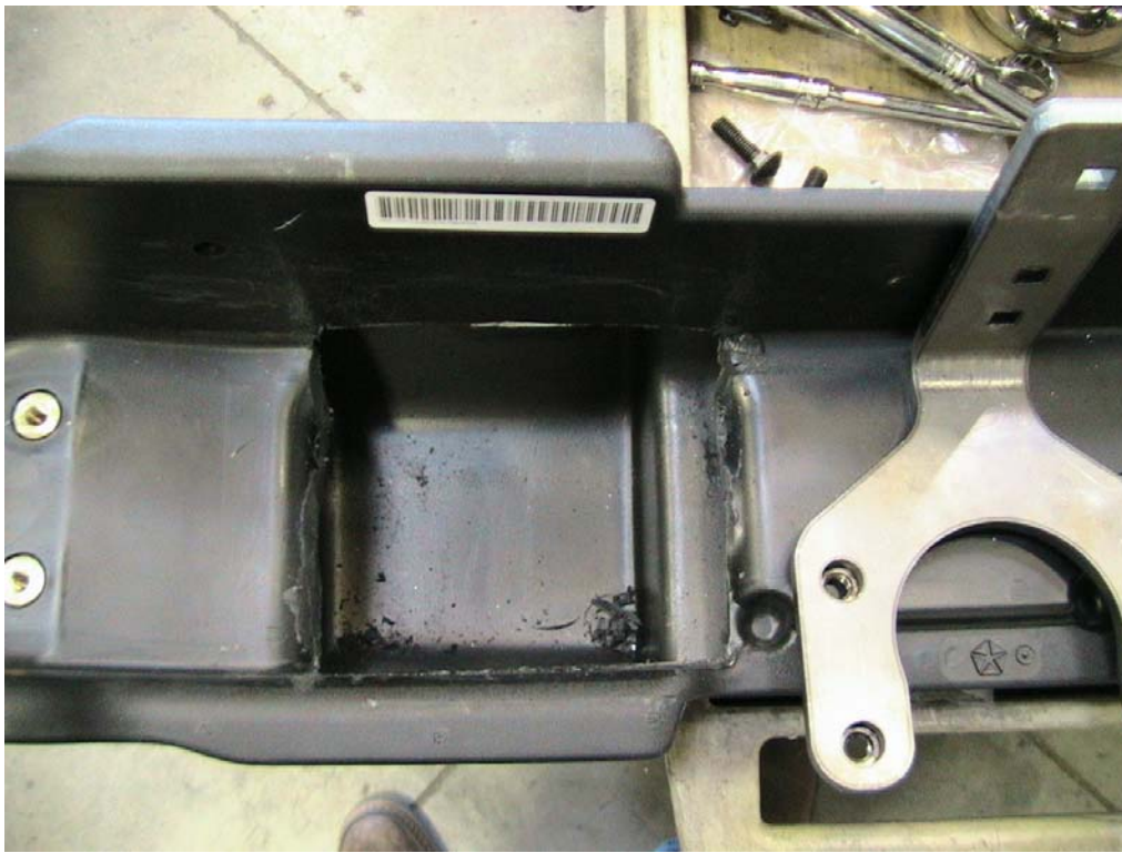
Figure 7: Cutout of inside of plastic bumper
