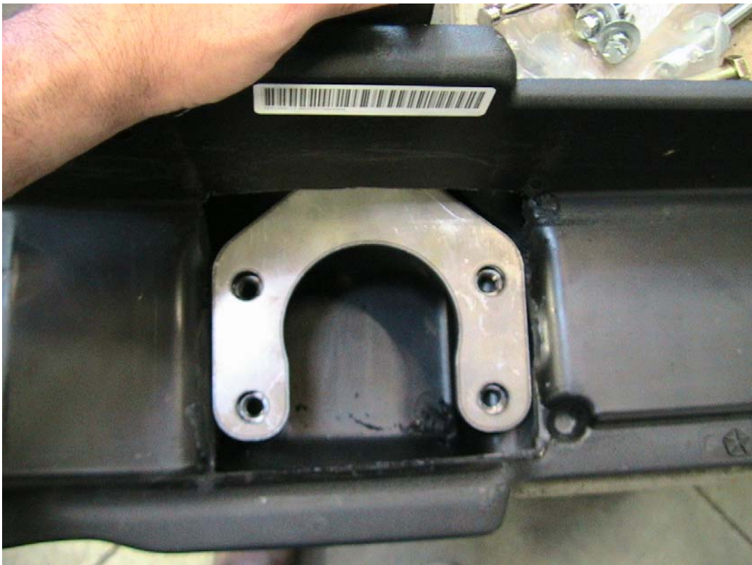
Figure 5: Tow hook fitment into plastic bumper
