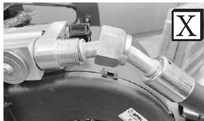
Improperly Seated O-ring Land
