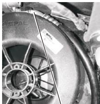
Connect 45° fitting on #6 A/C hose to corresponding port on evaporator
