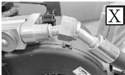
Improperly Seated O-ring Land
