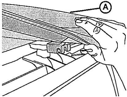
Place the Sunbonnet on the vehicle. Hook the body adapter on each side over the ledge of the door surround.
