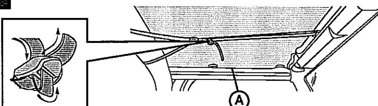
Thread the strap through the footman loop above the windshield. Pull the end of the strap back and thread it through the buckle. Pull it tight.
