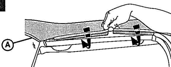
Roll the plastic strip above each door opening into the channel above the door on each side of the vehicle.
