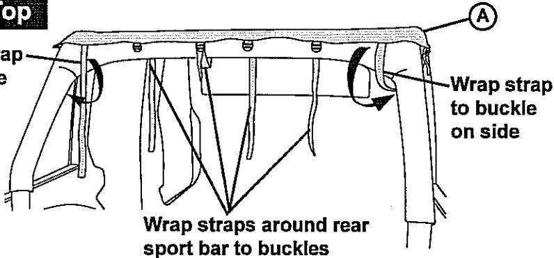
Wrap the straps on the rear of the Sunbonnet around the rear sport bar. Thread them through the buckles. Wrap the two (2) outside straps around to the buckles on the side.
