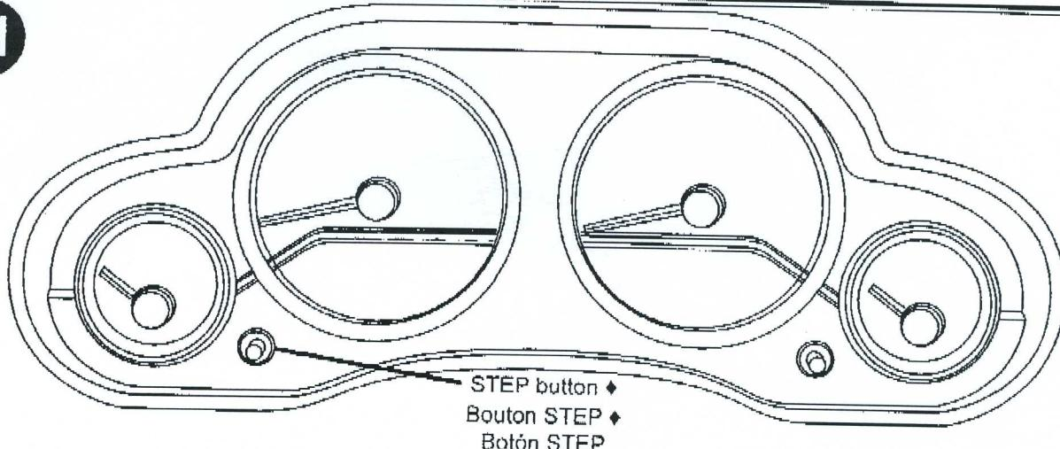
**EN** Manually calibrate the compass, as follows:
