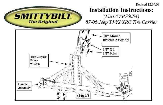
**<u>Step 13</u>**: Very carefully close the bumper and watch for tire carrier clearance over top of the bumper. *NOTE: Be careful not to scratch the top of the bumper.*
