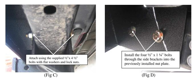
**Step 5:** Install the four ½" x 1 ¼" bolts through the side brackets into the previously installed nut plate.
