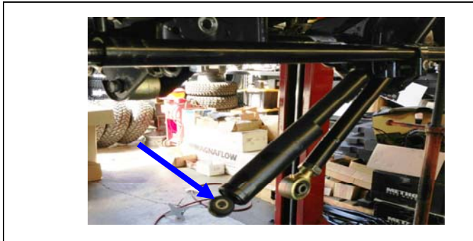
5. Remove the steering damper from the axle.
