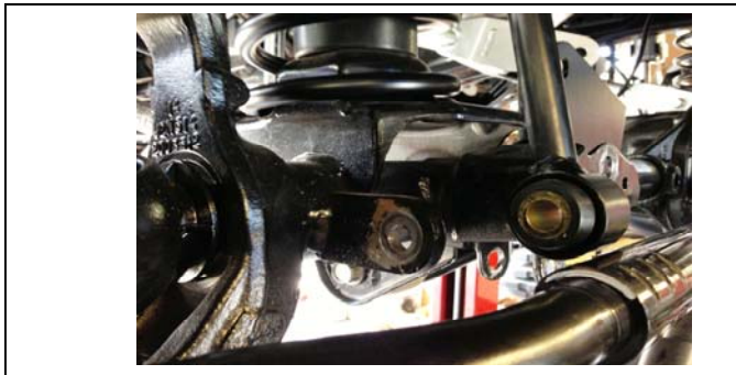
7. Remove the sway bar end links from the axle.
