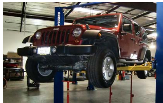
2. Lift the vehicle, supporting both the frame and front axle.
