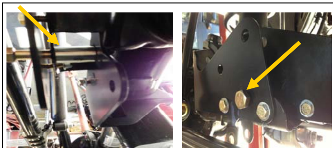
11. Insert the spacer in between the both brackets. Then tighten down all installed hardware and washers.
