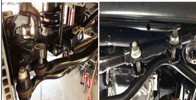
4. Remove the steering drag link from the axle, then loosen the coupler.
