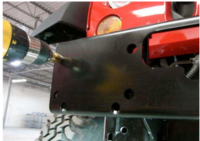
Drilling out the winch mount
