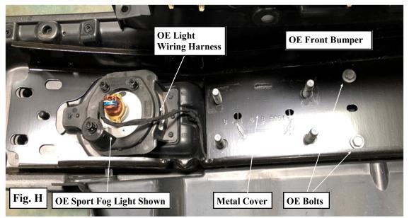
**Step 11:** Depress the locking tab and disconnect the connectors from the **OE** LED lights or **OE** sport fog lights. Save the **OE** wiring harness for reinstallation. (**Fig. H**)
