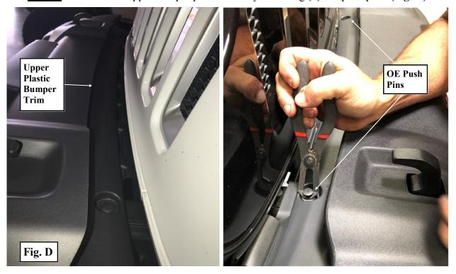
**Step 6:** Carefully remove the **OE** front bumper from the vehicle.
