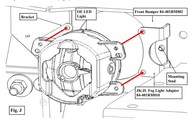
Step 15: Secure the OE LED lights to the JK/JL fog light adapter (84-401RM010) and the front bumper (84-401RM002 XRC) bracket using the (4 Per Light) provided 4mm X 16mm bolts and hardware. Make sure the OE LED light are centered in the window and tighten the mounting hardware. (Fig. J)
