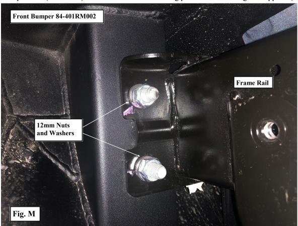
Per Side) 12mm nuts and washers. (Fig. M)
