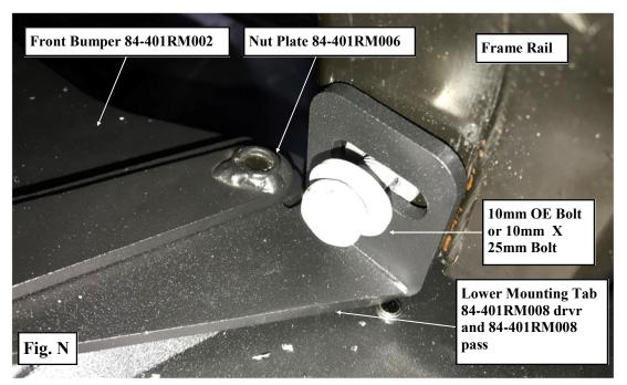
Step 21: Secure the (2 Per Side) front bumper lower mounting holes to the lower mounting tabs (84-401RM008 drvr and 84-401RM009 pass) using the supplied 8mm X 30mm bolts, washers, and nut plates (84-401RM006). (Fig N)
