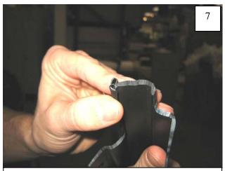
When positioning gimp on narrow end of rear, fold flat edge of gimp over the edge of the part. (Gimp will continue over entire length of part.)
