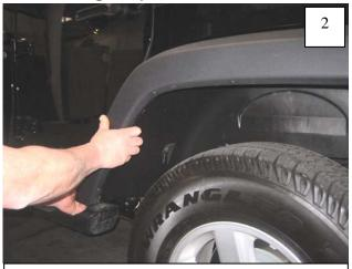
Starting at front of flare, pull firmly to release flare and splash shield from fender, working your way to the back. You will hear popping noises as clips release. It is O.K. if clips break, they will be discarded.
