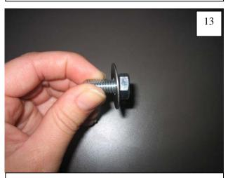
Position Inner Flare Piece on fender, aligning existing 5/16" holes in Inner Flare Piece with holes in fender. Slide a supplied 1" Fender Washer onto a supplied Hex Head Bolt.
