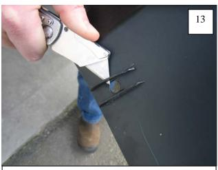
On backside of splash shield, use a utility knife to trim two plastic ribs flush with splash shield surface.
