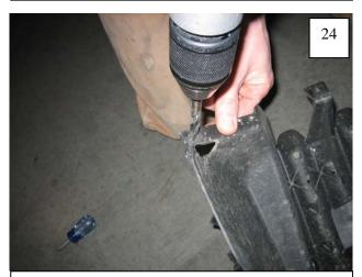
Drill one 5/16" hole in tab at forward area of splash shield as shown. The point of the drill should be approximately 5/16" down from top and 1/2" in from edge of tab.
