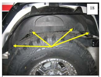
Install four supplied Plastic Phillips Head Tuf-Loks through splash shield and into vehicle body as shown.
