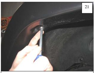
Install supplied Truss Head Screws through holes in wheel well and into #14 U-Clips installed in Step 15 (5 places).
