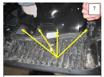
To remove inner structure and splash shield from factory flare, use a pry tool or flat head screwdriver to remove four plastic fasteners.
