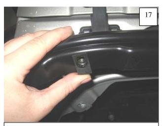
Install supplied Threaded Clips, with the thread side in, over holes in Inner Flare Piece (8 places). Make sure clips are centered over holes.
