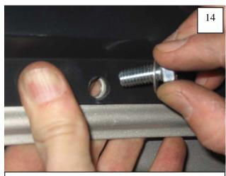
From inside of fender, hold a supplied 1" Fender Washer over hole. Insert a Bolt/Washer assembly through Inner Flare Piece, fender, and washer on backside of fender.
