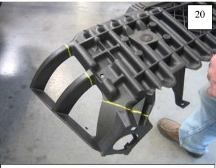
Draw a line from the corner of the cut out diagonally across the ribs of the factory inner structure as shown. NOTE: Line placement can vary 1/2" inch in either direction from shown.
