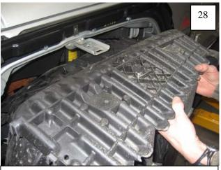
Replace factory inner structure/splash shield in fender as shown, sliding hole in structure over metal fender bracket.
