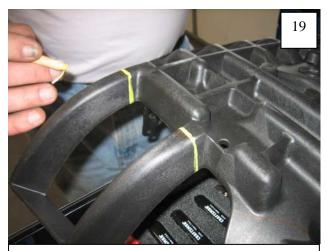
Using a grease pencil, trace a line along the base of the first and second spines of the factory inner structure as shown. This line will be cut in Step 21.
