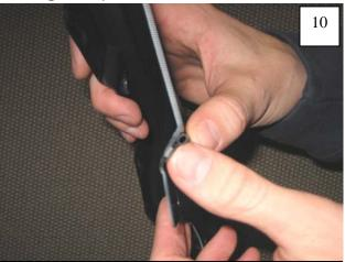
Make sure gimp and inner flare are clean. Peel 2" of liner from gimp (pin shape). Carefully position gimp as uniformly as possible along radius as shown, peeling liner as you go. Gimp can be repositioned as needed. NOTE: it is better for gimp to be slightly below radius rather than above.
