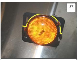
Carefully cut or grind factory light bezel along lines shown. Take care not to cut light lens.
