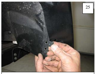
Pull the splash shield out from behind flare and install a supplied #14 U-Clip over hole drilled in Step 23. This hole will be located slightly above existing hole in splash shield.
