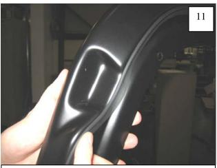
When positioning gimp around latch section of front, make sure round edge of gimp is positioned below the edge of the part. (Gimp will continue over entire length of part.)
