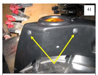
Install supplied Plastic Phillips Head Tuf-Loks (2 places). Use a pushing-twisting motion to install. Gently pull tab to peel tape liner from 1/2" tape and press in to place.
