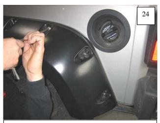
Remove three rearmost screws installed in Step 20.
