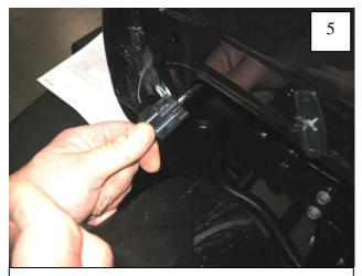
Once flare is free of fender, disconnect light connector. This will allow the flare to come away from fender completely. Remove light housing from factory flare; you will be reinstalling this later.
