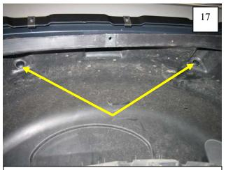
Position splash shield in wheel well, and install two supplied Plastic Phillips Head Tuf-Loks in upper pockets using a pushing-twisting motion.
