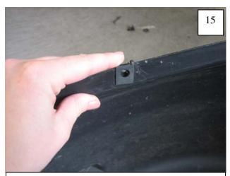
Install supplied #14 U-Clips over existing holes in splash shield (5 places). Flat side will be visible once splash shield is reinstalled.
