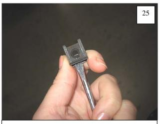
Use a flat head screwdriver to spread supplied #14 U-Clips for ease of installation.
