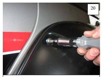
Start Screws/Washers through pocket holes in flare and into Threaded Clips installed in Step 11 (8 places) starting at the front and working your way to the back. Do not tighten.
