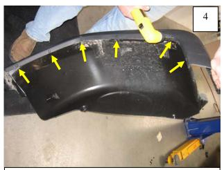
Use a drill with a 5/16" bit to drill through six plastic rivets along edge of flare/splash shield. Discard the flare, but retain the splash shield. NOTE: It is helpful to angle the drill while drilling the rivets.
