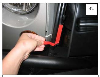
Fold tape liner tab attached to 1/2" piece of tape on outer edge of Inner Flare Piece upwards (do NOT peel liner from 1/2" tape in this step).
