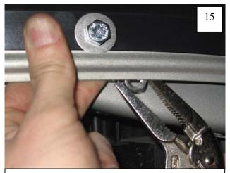
Using a vise grip, place a supplied Nylock Nut on the backside of the Bolt. Start bolts but do not tighten (8 places). Once all bolts have been started, tighten all bolts.
