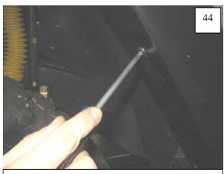
Install supplied Truss Head Screws through holes in wheel well and into #14 U-Clips installed in Step 25 (6 places). Ensure proper alignment of outer flare, inner flare, and splash shield. **Do not tighten.**
