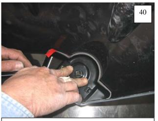
Place Light Pocket Inner Piece with light bezel into inside of Front Flare, aligning light lens with hole in flare. NOTE: Make sure tape liner is protruding from part for ease of liner removal.
