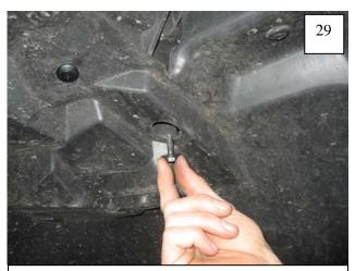
Reinstall the factory bolt in hole in splash shield as shown.
