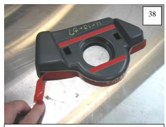
Peel liner completely from two pieces of 1/4" tape located on face of Light Pocket Inner Piece. Fold tape liner tab attached to long 1/2" piece of tape upwards (do NOT peel liner from 1/2" tape in this step).
