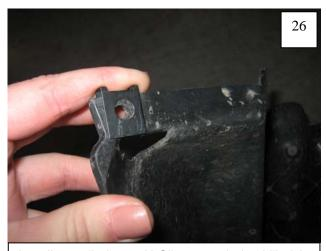
Install supplied #14 U-Clips over hole drilled in Step #24 and five existing holes in splash shield.
