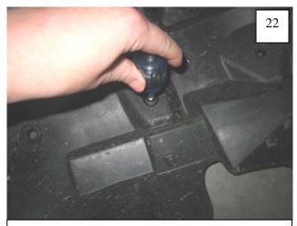
Using a Phillips screwdriver, reassemble inner structure and splash shield by installing supplied Plastic Phillips Head Tuf-Loks (6 places). Use a pushing-twisting motion to install.
