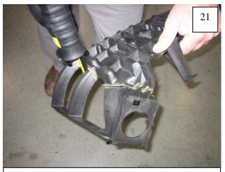
Using a hacksaw or SawsAll, carefully cut along lines made in Steps 19 and 20 to remove from portion of factory inner structure. Retain rearward piece.
