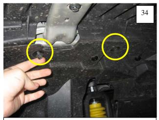
Reinstall two factory bolts as shown.
