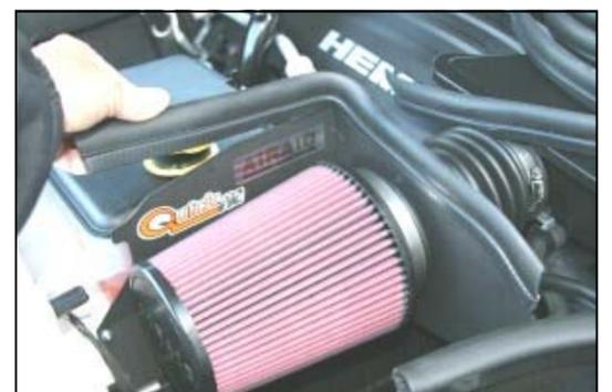
**9. Install the weather strip (#4) onto the top of the Quick Fit Panels. (Hint: For ease of installation, start at one end and work your way to the other).**
