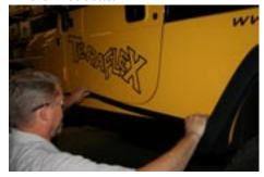
11. Drill final holes through the weather stripping and the body using the five holes located on the rock slider.
