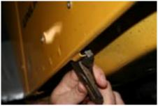
4. Lay down some tape both on the fender flares and the inside of the rock slider to protect the body while lining up the rock sliders for installation. Remove the tape before final installation.
