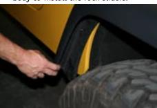
2. Remove the lower front fender flare. It is a separate piece from the front fender flare.
