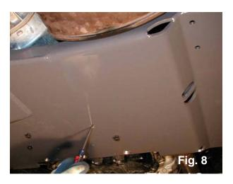
**Step 11:** Adjust T-case linkage. Even though the t-case linkage relay rod position has been corrected for the TT installation, you will still need to re-adjust the linkage for proper t-case shifting. Begin by
