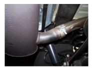
2. To remove the stock exhaust, unbolt band clamp located just behind your factory muffler. Disengage the welded hangers using WD-40 from the OEM rubber grommets. Do not damage or remove the rubber grommets as you will reuse them to mount your new system. Now, cut off tailpipe and remove exhaust.
