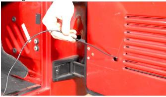
Reinstall the air vent and secure the rest of the Backside to the tailgate.
