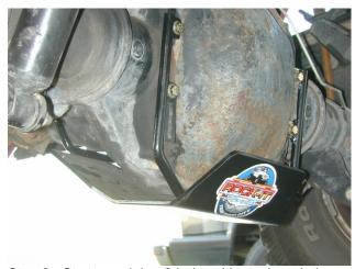
Step 3: Start remaining 2 bolts with washers in lower Glider Bracket. Do not tighten.
