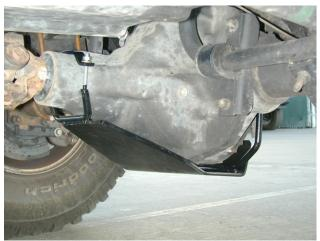
Step 4: Place retainer strap on studs over top of pinion area of differential. Start 2 nuts and washers to secure rear of Glider as show
