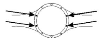
Step 1: Remove 4 original cover bolts as shown.
