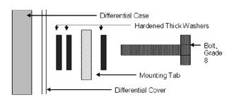
Step 2: Start 2 upper bolts with provided hardware as shown. Use 2 thick washers as spacers behind Glider Bracket. Do not tighten yet.
