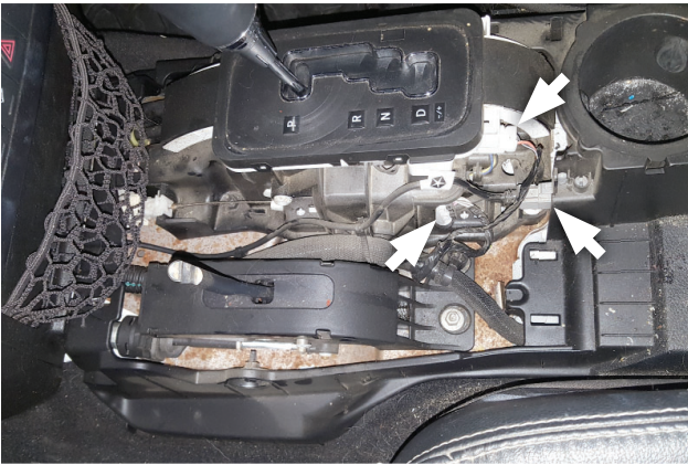
7. Disconnect wiring connectors from shifter and console.
