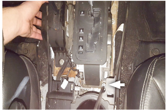
10. Lift console to unhook tabs, move it aside then remove and retain remaining nut from shifter.
