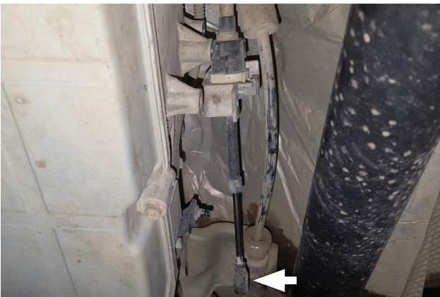
14. Remove shifter cable from transmission as shown.
