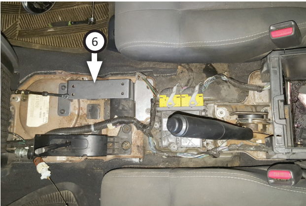
25. Fasten mounting bracket (6) to shifter location using nuts (x4) (removed step 9).
