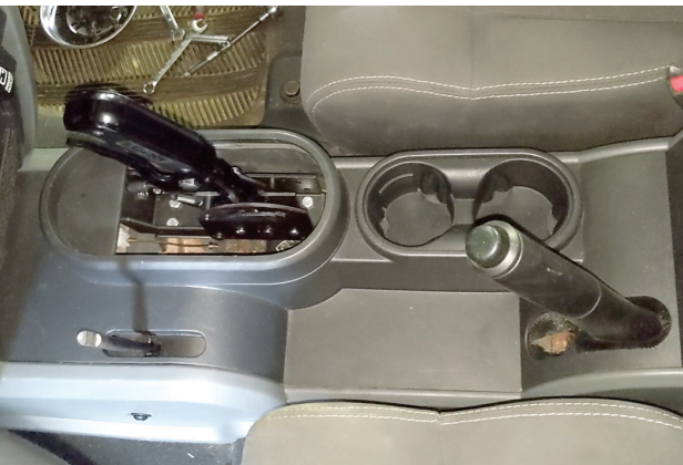
31. Install console case (removed step 6) using fasteners (x10) (step 5), then install console top (step 4).
