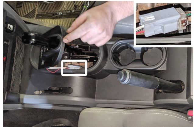
33. Connect console cover connector to factory cable but do not close console cover yet.
