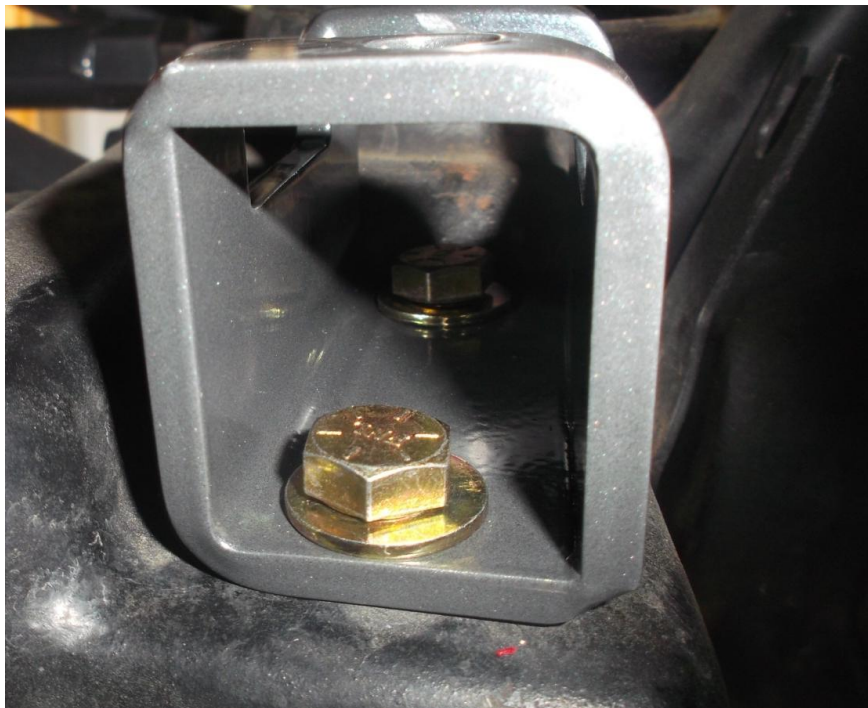
Figure 4. Shock Extensions Installed With Bent Edge on Right, Facing Tire
