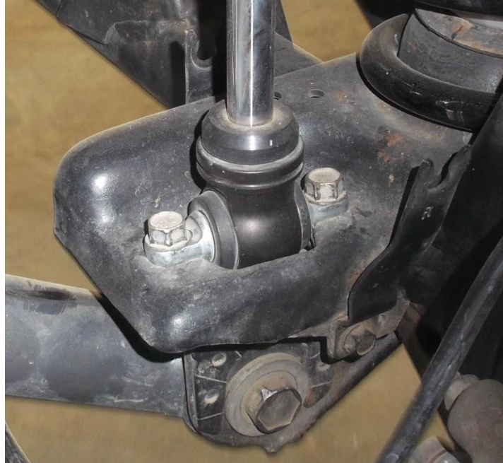
Figure 1. Lower Shock End in Axle Bracket
