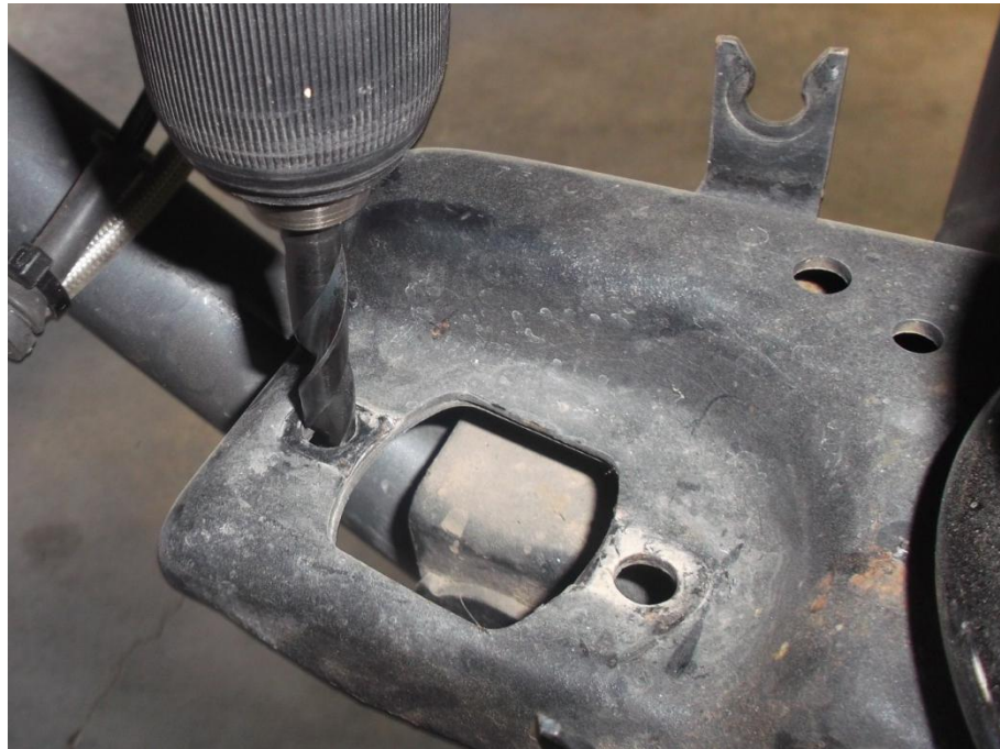
Figure 2. Drilling Out Shock Mounting Holes
