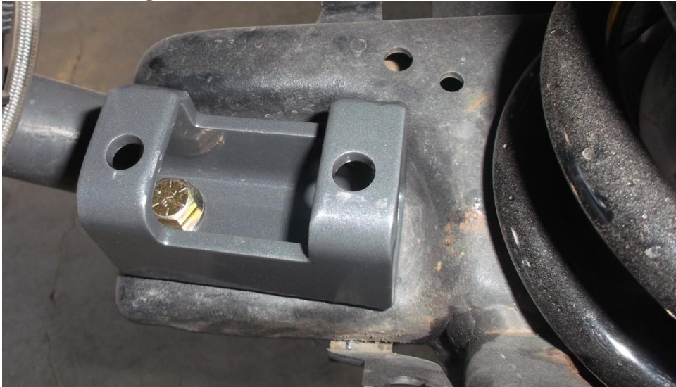
Figure 3. Shock Extensions Installed With Opening Facing Up, Bent Edges Out
