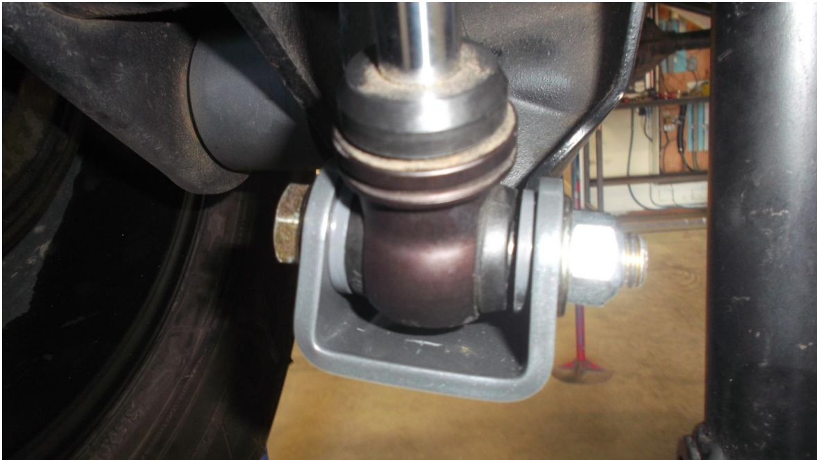
Figure 4. Spacer Washers Correctly Installed
