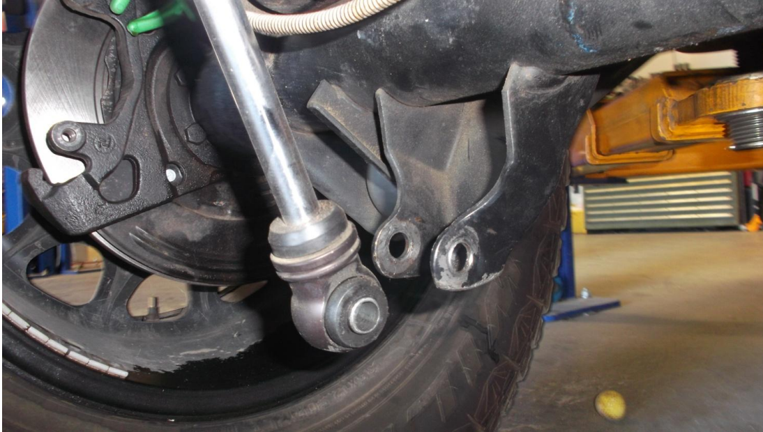
Figure 1. Lower Shock End Removed from Axle Bracket
