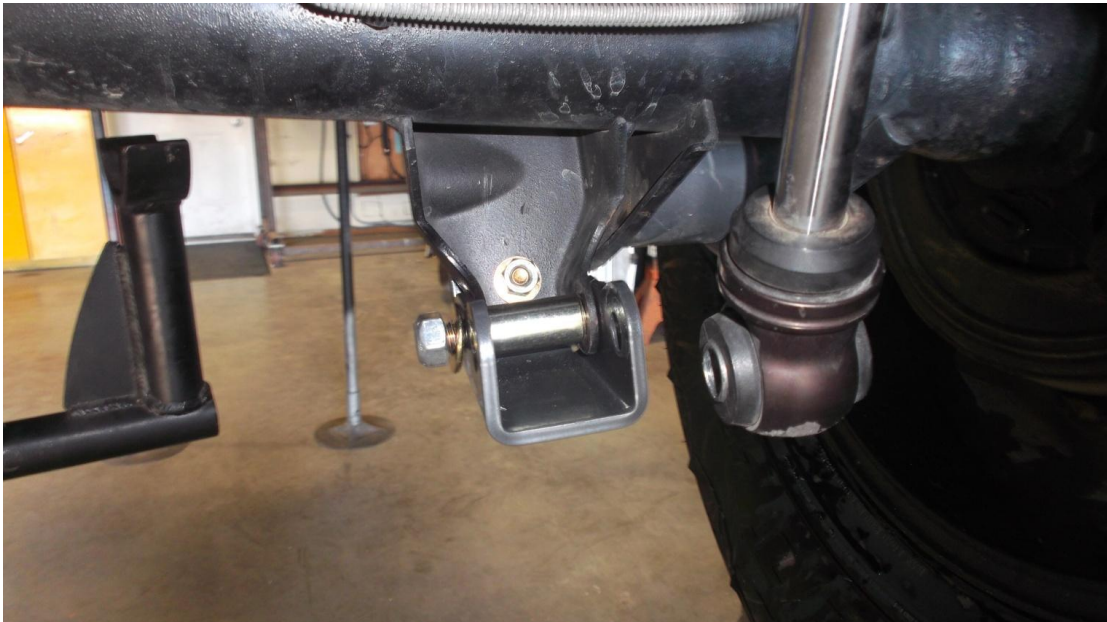
Figure 2. Synergy Shock Relocation Brackets Installed
