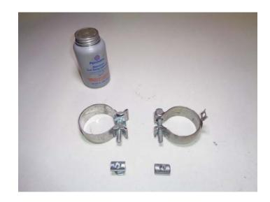
13. Place factory clamp (removed step 11) over ball end of factory inlet. Mate ball end of muffler (815425-516) to factory pipe and tighten factory clamp just enough to allow for adjustment. Slip clamp (MC250BS) over muffler outlet.
