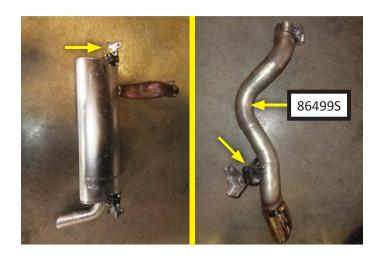
8. Remove stock resonator assembly from rubber isolator with a pry bar and retain for re-use.
