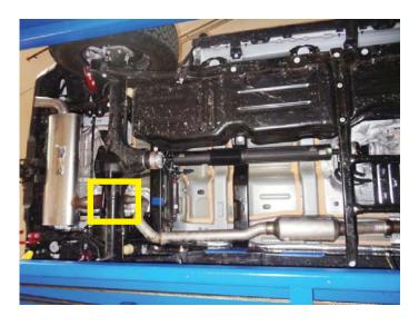
6. Remove muffler from vehicle.
