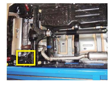
4. Remove bolts (x2) from mount on passenger side above muffler in area indicated.
