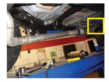
10. Remove resonator assembly from vehicle.
