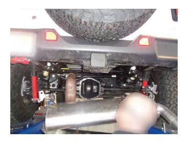
7. Place stock muffler next to tailpipe **(86499S)** oriented in the same direction. Then transfer driver side mount from muffler to tailpipe.
