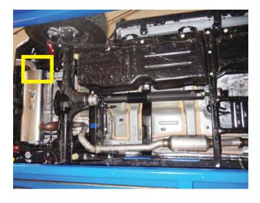
5. Loosen clamp at muffler inlet connection above rear axle.
