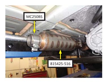
14. Place **front inlet pipe (86505S)** into muffler. Make sure bend on front inlet pipe is oriented upwards for maximum clearance (as indicated). Tighten clamp just enough to allow for adjustment.
