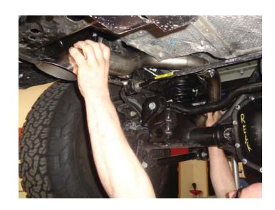
17. Place factory (driver side) mount into position, then reinstall and tighten factory bolts (x2) (removed step 3).
