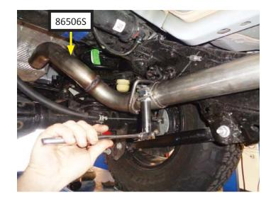
16. Place **clamp (MC250BS)** onto slip-fit of tailpipe, then slide tailpipe onto rear inlet pipe. Make sure tailpipe bend curves over suspension components then ensure connections are completely seated.
