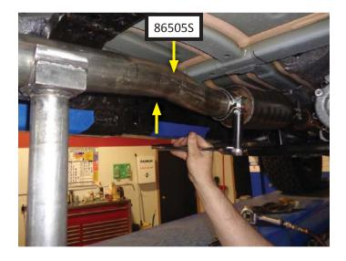
15. Place clamp (MC250BS) onto slip-fit of rear inlet pipe (86506S). Connect front and rear inlet pipes while pushing wire hanger into rubber isolator on vehicle. Tighten clamp just enough to allow for adjustment.
