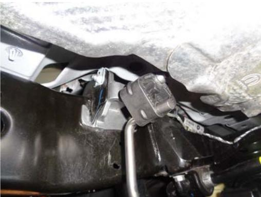
2) Place the factory hanger mounts back into position and secure them to the frame using the factory bolts, tighten securely.
