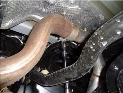
2) Using a 15mm socket, loosen the clamp at the muffler inlet connection above the rear axle.
