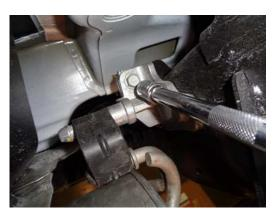
4) Then, use a 13MM socket wrench to remove the upper bolt on each mount. Once both hangers are un-fastened, carefully lower the stand and with the help of an assistant slide the muffler off of the inlet pipe and remove from the vehicle.
