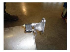
5) Place the factory muffler next to the new Flowmaster muffler and move the factory hanger mounts onto the wire hangers of the new muffler.
