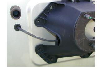
3 RUN CABLE ALONG WITH OTHER WIRES IN HARNESS
