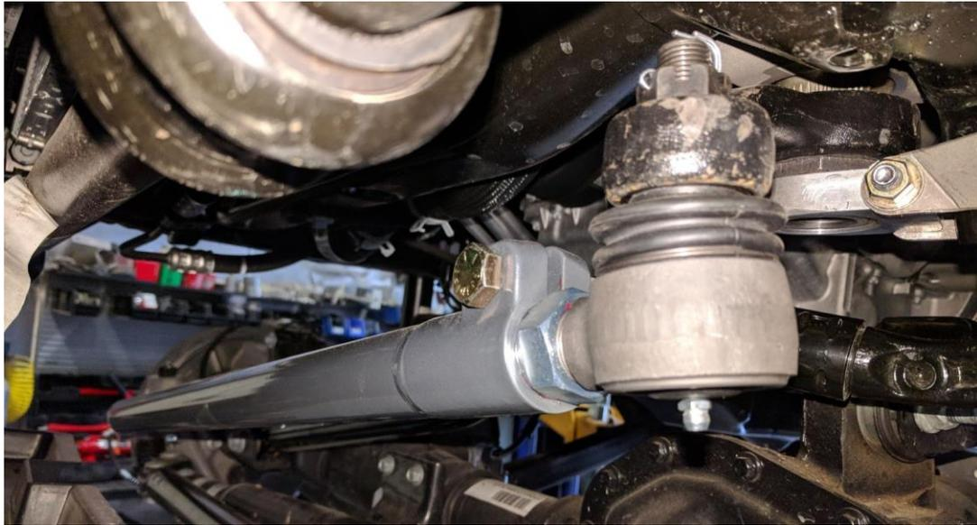
**Figure 7. Drag Link Correctly Oriented, Pinch Bolt Up**
