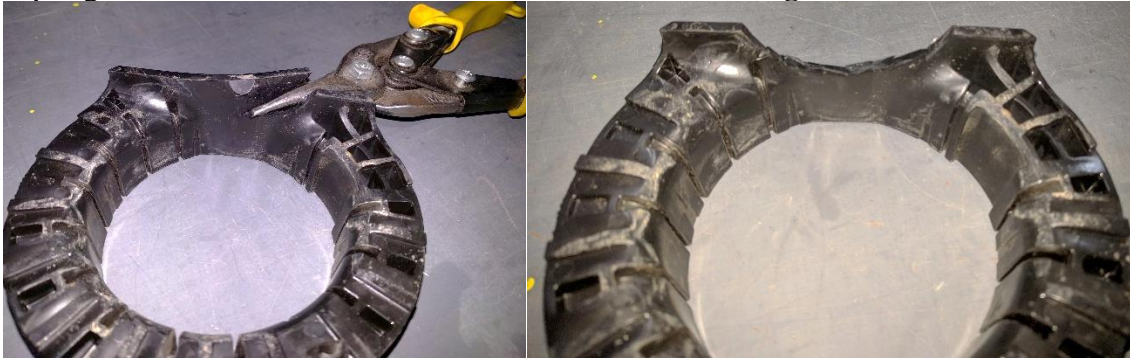
Figures 7 and 8. Trimming Stock Lower Spring Isolator
