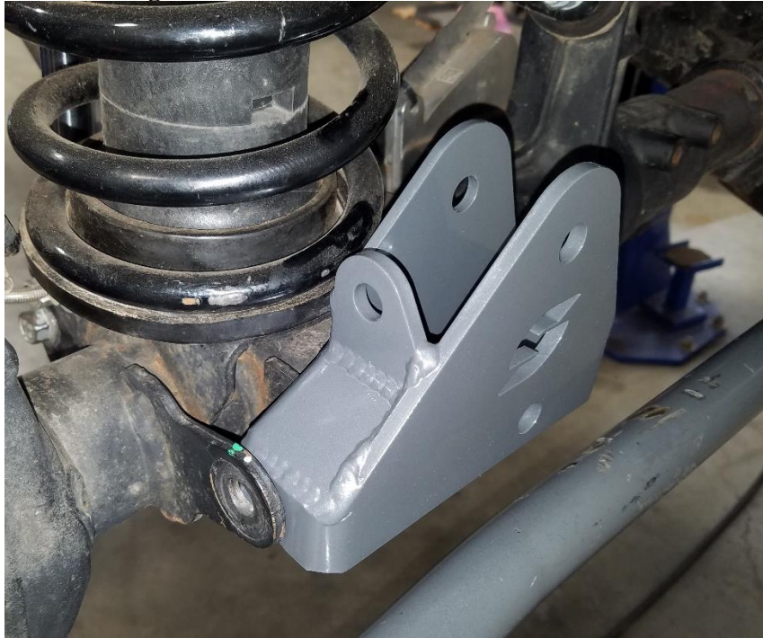
Figure 2. Synergy Bracket Loosely Installed
