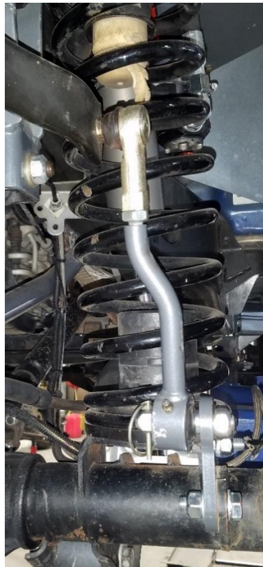
Figures 11. Correctly Installed Driver's Side Sway Bar Link
