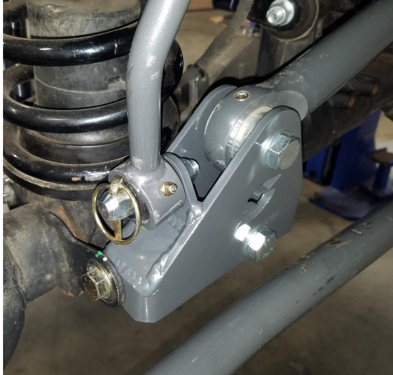
Figure 12. Sway Bar Link Installed on Bracket
