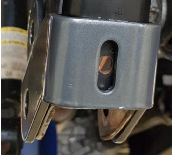
Figure 1. Hole drilled for rear shock relocation.
