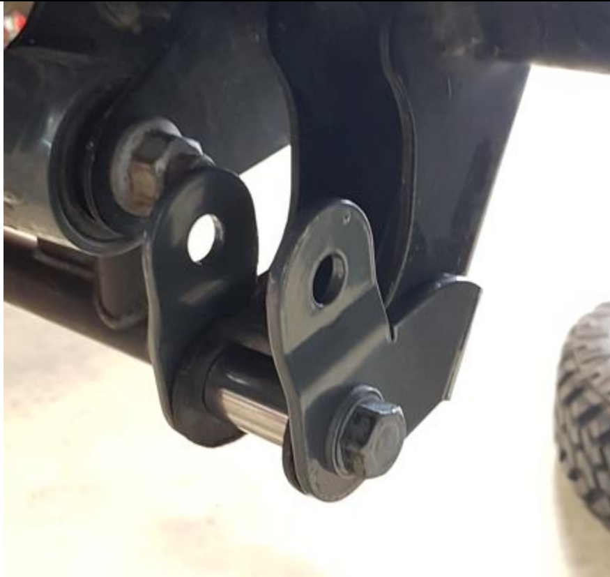
Figure 3. Bracket and spacer installed
