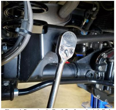
Figure 1. Removing the Track Bar from the Axle End
