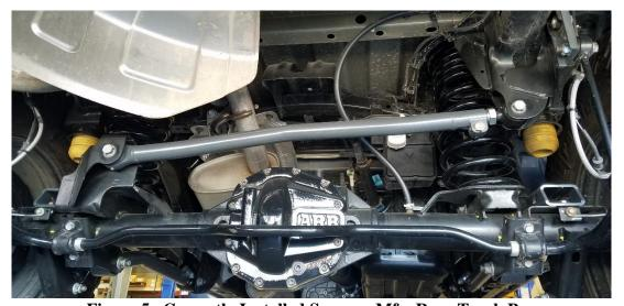
Figure 5. Correctly Installed Synergy Mfg. Rear Track Bar
