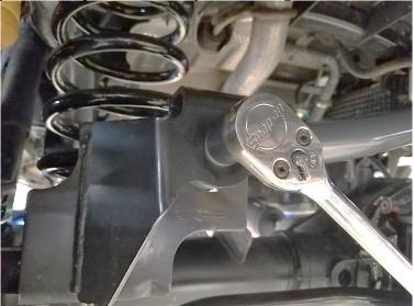
Figure 4. Installing the Synergy Mfg. Track Bar at the Axle
