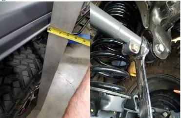
Figure 6. and 7. Measuring Side to Side and Adjusting the Track Bar to Center the Axle
