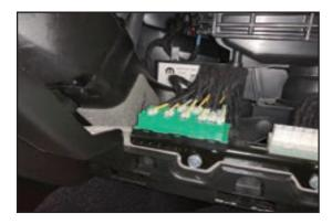
11. Take the supplied bypass cable shown and connect the white connector as shown at the red arrow location. Route the cable along the base of the dash towards the OBD connector. Use zip ties to secure it out of the way.
