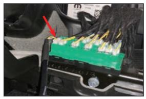
12. Plug the end of the supplied connector into the ODB port. (The other end will be used when flashing with the RTD device.)
