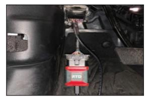
13. For 2012-2017 vehicles plug the RTD directly into the ODB port.
