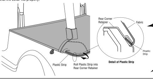
Note: The Plastic Protector sewn into the fabric must be located over the ends of the Tailgate Bar.
