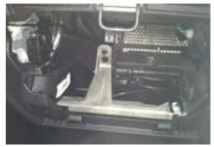
**Step 27:** Using a plastic trim removal tool, remove HVAC panel.
