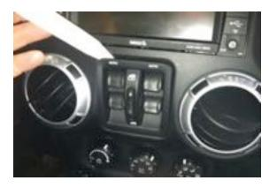
Step 21: Disconnect harness from window switches.
