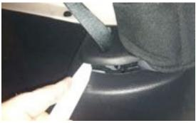
**Step 12:** Using a plastic trim removal tool, remove rear access panel to expose 10mm bolt, and remove bolt.
