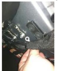
Step 18: Remove rubber bin insert from top of dash.
