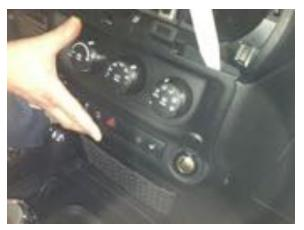
**Step 28:** Run Red 12v+ ignition power wire and green trigger wire of supplied Chassis Harness to ignition controlled power point on HVAC panel power point.
