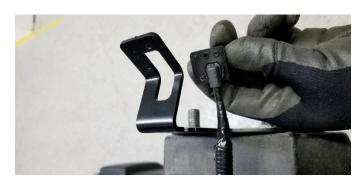
**Step 2:** Line the mounting holes from the new brake light bracket up with the mounting holes of the Camera and mounting bracket and reinstall the two #1 Philips screws.
