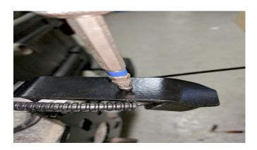
**Step 2:** Line the mounting hole from the new brake light bracket up with the mounting hole of the Camera and mounting bracket and reinstall the one #1 Philip screws.
