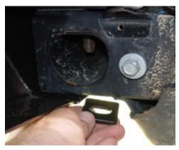
Step #7: With the top OE bolts in place install the lower OE bolts. (Insert lower spacers if needed)
