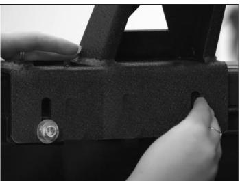
Step 2. Place the Cargo Rack on the proper position. Install two Side Cargo Rack onto the nut plate just installed using the supplied M8x30mm Allen head bolt and M8 flat washer.
