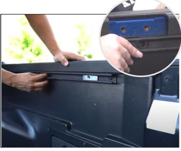
Step2: Slide 2 nut plate in the rail. Don't have to position it in the exact location just yet.
