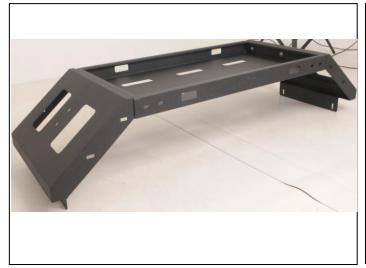
Using a blanket on a table or the ground. Assemble the Cargo Rack together using the supplied M8x20mm button head bolt, flat washers, split washer and M8 nuts.
