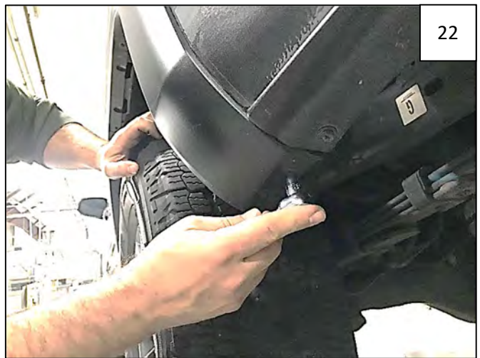
Remove 1 factory screw from underside of factory flare at rear.
