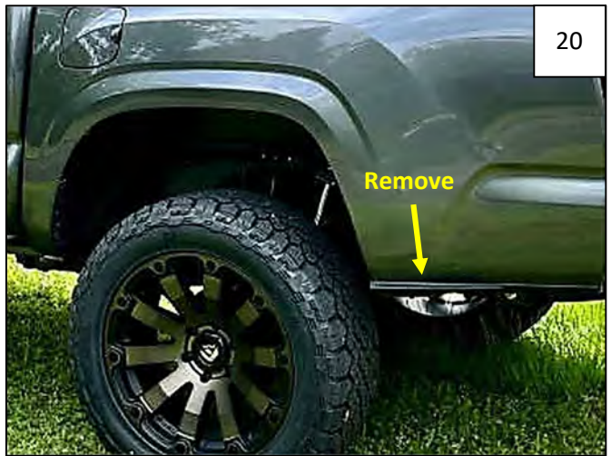
If your vehicle does not come with factory flares, the trim piece located at the rear must be removed – this part will interfere with flare installation. If flares are present, skip to Step 18.
