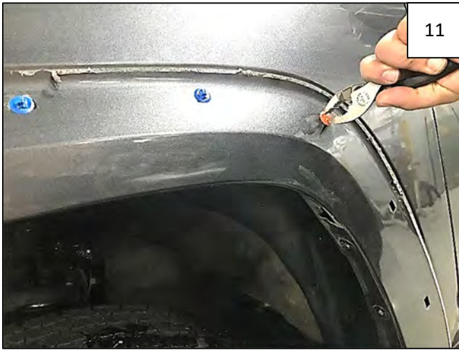
11 Use a vise grip or pliers to remove 1 factory clip as indicated by circle in Step 10, pulling with a rocking motion.
