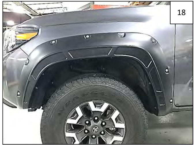
Complete Front Flare Installation.
