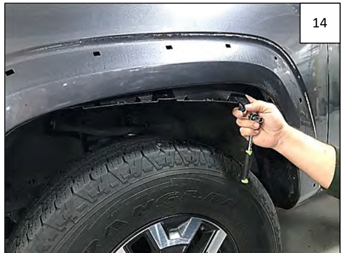
14 Line 3 holes in Inner Bracket with 3 uppermost holes in fender. Start 3 supplied 20mm Hex Screws through Inner Bracket and into holes in fender. Tighten screws.
