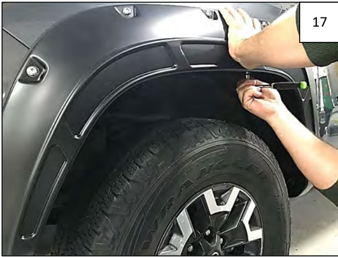
Apply pressure to flare towards vehicle body at each fastening point and tighten all fasteners.
