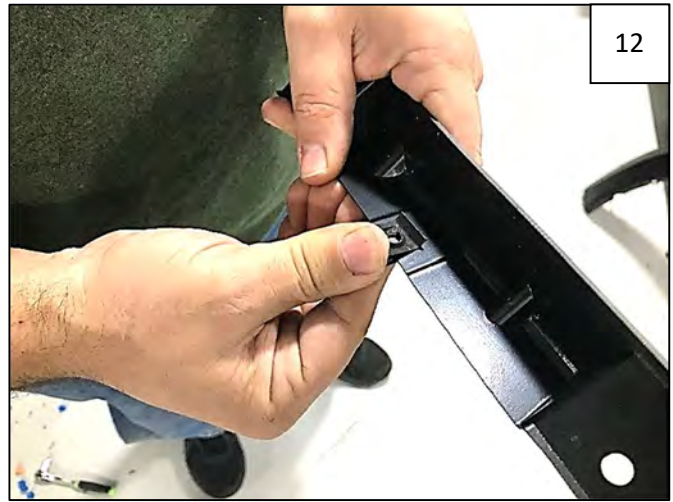
12 Attach 2 supplied #14 "U" Clips to supplied Inner Bracket as shown. Left Front Bracket is marked as "LF" and Right Front Bracket is marked as "RF"
