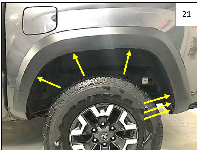
Remove 6 factory screws from factory flare as indicated by arrows. NOTE: If no factory flare is present, skip to Step 26.
