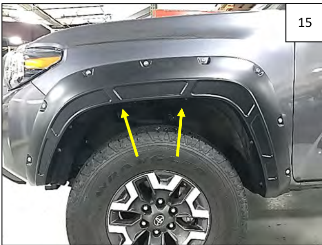
15 Aligning flare on fender and pressing toward vehicle, start 2 supplied 20mm Hex Screws through flare and into clips installed on Inner Bracket.
