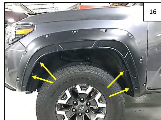
16 Install 4 supplied 20mm Hex Screws through remaining holes in flare and into holes in fender.
