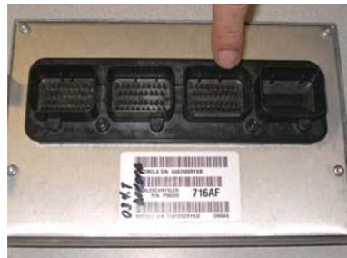
Step 4: Lay your computer on a flat surface and plug your Jet Module into the connector shown in the pictures above and below. Be sure the module fully seats or the vehicle may not start. Now with the module installed in your computer, mount the computer back in the vehicle and plug all the wiring harness plugs back into you computer and the Jet Module.
