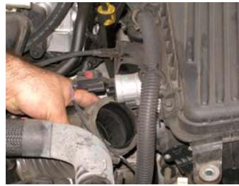
Step 3: There are four connectors located on the front of the computer. Disconnect all four connectors from the computer by pressing down on the release buttons on each wiring harness plug. Next remove the three bolts holding the computer to the vehicles body.
