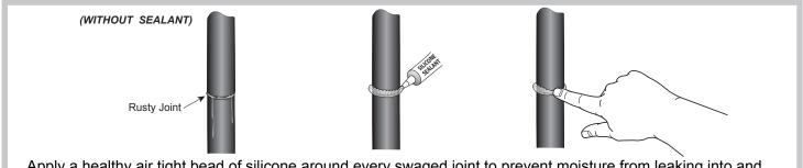
Apply a healthy air tight bead of silicone around every swaged joint to prevent moisture from leaking into and out of the joint. If this is not done properly, the inside surface of the tubes can rust and rusty water can leak out. Maintain this joint seal throughout the life of your rack.
