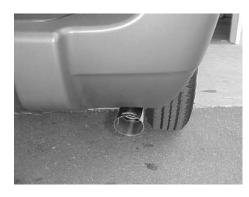
**INSTALL YOUR** STAINLESS TIP TO YOUR DESIRED LOOK. TO CLEAN TIP LISE ANY ALUMINUM OR **STAINLESS** CLEANER AND A SCOTCH BRITE PAD. NOW TIGHTEN ALL CLAMPS STARTING FROM THE FRONT AND WORKING BACK.
