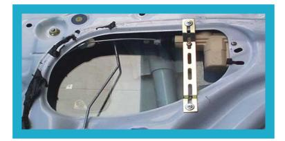
Notice how this actuator is partially fastened to the door and to the strap. You should be clear on the fact that the attachment is not as critical as the placement. Just make sure that the actuator is attached securely, and does not interfere with any other mechanism. Whenever installing an actuator inside the metal panel, extreme care should be taken with regards to window movement.
