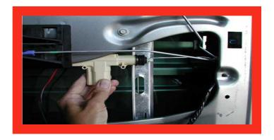
This photo shows placement of the actuator in position prior to fastening. The vehicle in the photo is a 2000 Chevy Silverado. Photos and installation compliments of A-1 Electric. A-1's installer will use the strap that is supplied in the Electric-Life door lock kit to span the hole in the door and permanently fasten the actuator in place.
